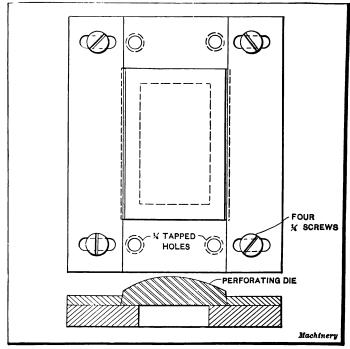
Fig. 13. Device for Holding Perforating Dies while Filing
